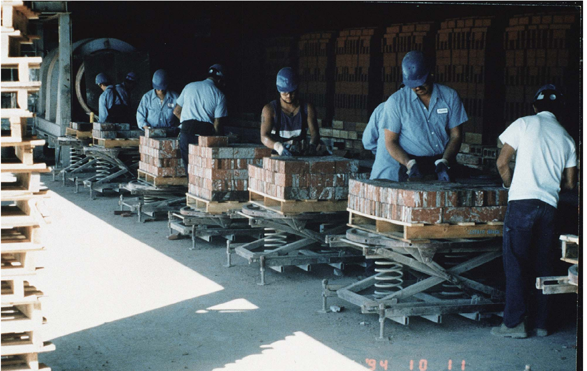
The Southworth PalletPal at work... Notice the level load surface despite varying load weights. The product being packed is bricks!
