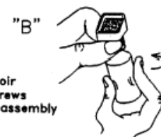
"B" hold reservoir assembly, ink pad up grip bottle cap / untwist bottle fill and reverse procedure to re-install
