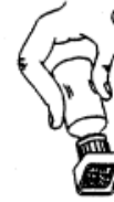
6. "Quick start" ink by squeezing bottle until ink saturates pad and release to remove excess ink.
