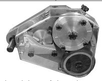
with special adaptations for horizontal operation. A control enclosure, motor and special ink fountain have been added
