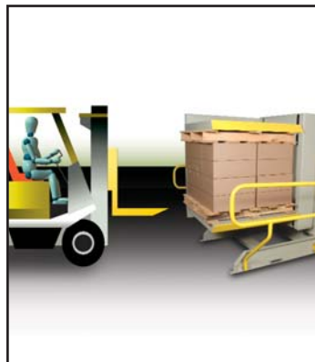
2. Place loaded pallet into inverter.
